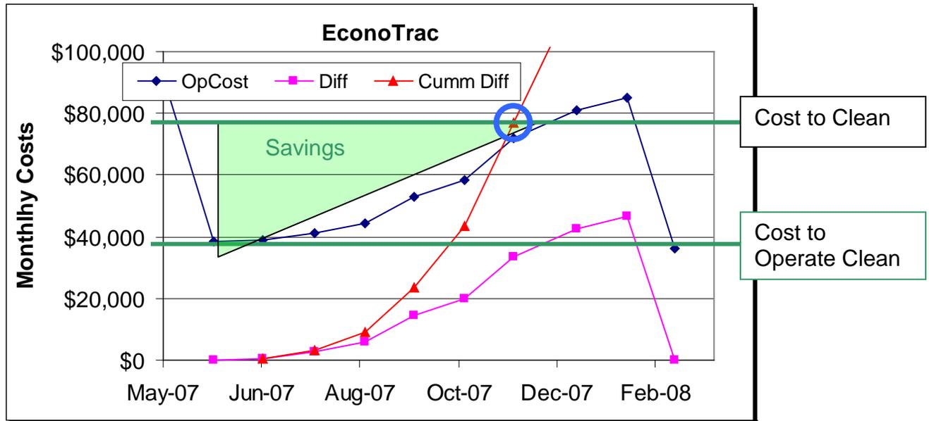
Organic re-fouling starts right after the cleaning, of course, but in most cases it takes a few months for the fouling to build up to the level where it impacts on the operation. When that occurs, the monthly costs will start to rise, eating into the savings. The key metric we use now is the cumulative increase in operating costs, representing the total increase in costs month by month over the base case. This is the red line, and it rises at an accelerating pace.
