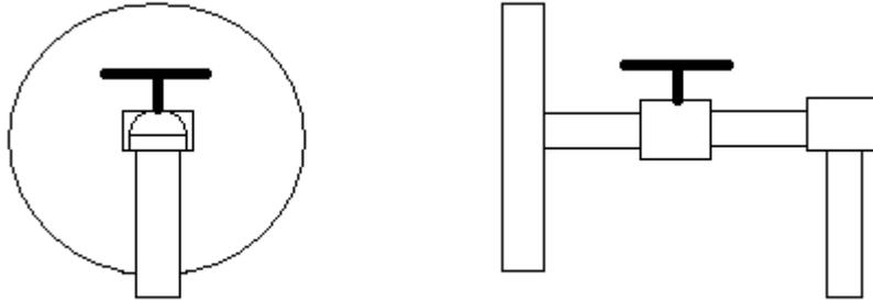
The sampler replaces the blind flange normally sealing the resin removal port. The valve depicted above is a lockable ball valve. The lock is needed to prevent accidental opening of the valve while the unit is on-line; this would allow resin to quickly flood from the vessel onto the ground. The samplers should be made out of stainless steel.
