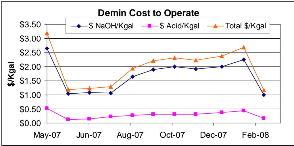
Note the gradual rise in the cost to purify 1000 gallons of water, after an initial delay. This is the direct effect of organic fouling.
