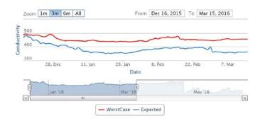
**Throughput**, based on the projected conductivity combined with the expected resin capacity from the salt split curve. In this case, with and without resin cleaning are compared:
