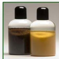
*To the left...fouled Ion Exchange Resin prior to restoration*
